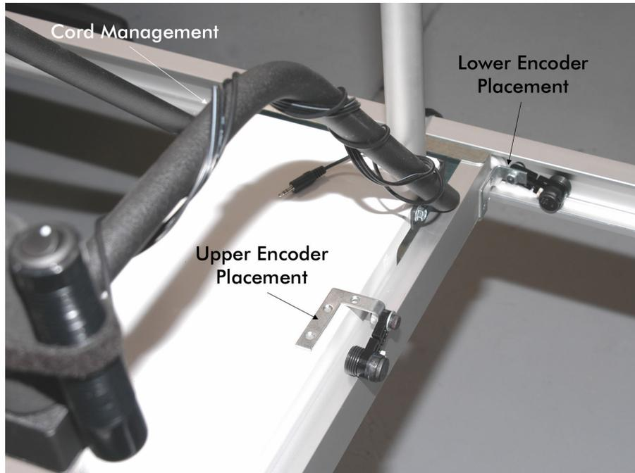
The photograph shows the overall placement of the optical encoders on the quilting frame carriages. Please follow the detailed installation instructions in the user manual to complete the installation.
